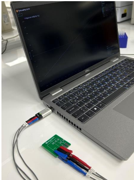
Figure 14. Connecting a Banana Interface to the GalvanoPlot Instrument via PC USB Port.
